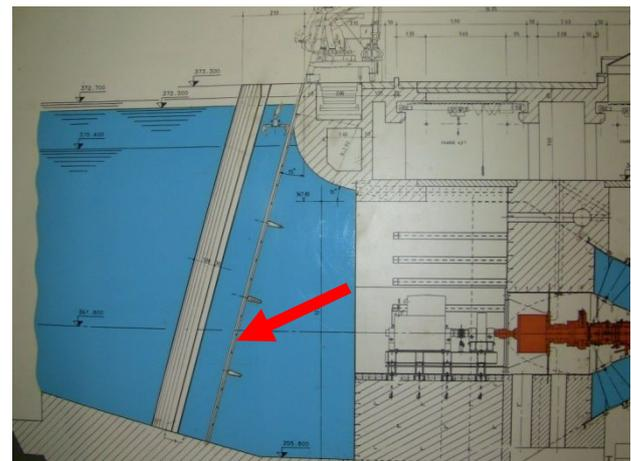
Figure 2: Cross section view of the dam and the turbine. The grid is marked by a red arrow.
